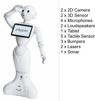
Fig. 1. Peppers Sensors: A list of the most useful sensors for human-robot interaction
