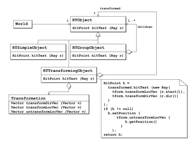
1c) <u>Task</u>: When transforming an object it is typical to construct the transformation from the basic transformation scaling, rotation, and translocation by putting them in a sequence of transformation operations. Extend the class structure to represent such sequences of transformations. Discuss different solutions.
