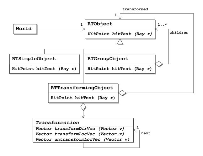
If we change this slightly by having the RTTransformingObject invoke each elementary transformation in the sequence instead of passing the call from one transformation to the next, we can even pre-process the transformation chain and optimise its performance by condensing it into a single transformation.
