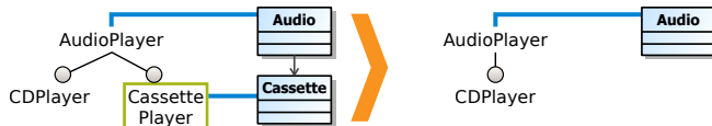
Figure 2: Example of Remove Feature and Owned Assets to delete the feature CassetPlayer and its implementation.
