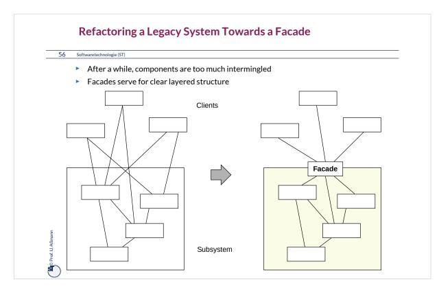
One of the most important restructuring operations in old systems is to introduce modules, subsystems, or packages by encapsulating them by a facade object.
