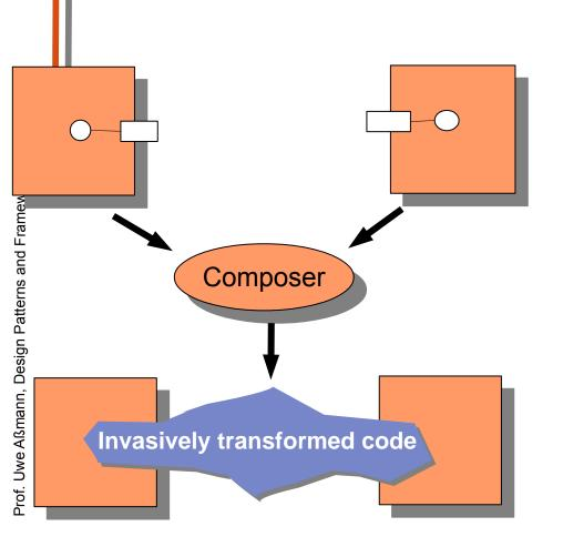
Invasive Composition adapts and extends components at hooks by transformation (2-level composition algebra)
