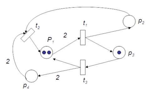
A PN with initial marking  $(2 \ 0 \ 1 \ 0)^{T}$ . The state equation is shown, where  $t_3$  fires to result in  $M_1 = (3 \ 0 \ 0 \ 2)^{T}$ .
