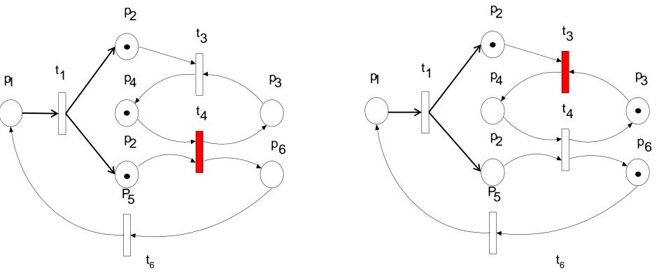
p2 is a synchronization dependency; process p5 can run earlier, p2 has to wait. Note: the content of p2 must be reproduced again Net is unbounded, due to the reproduction facilities of t6
