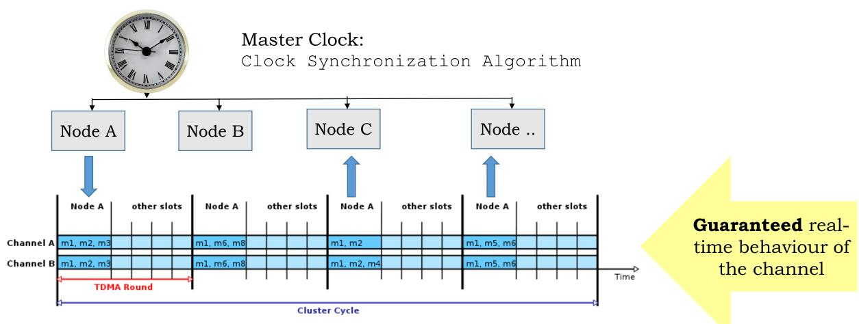
The messages are transported in exactly defined and assigned time slots, based on precise clock synchronization in all nodes
