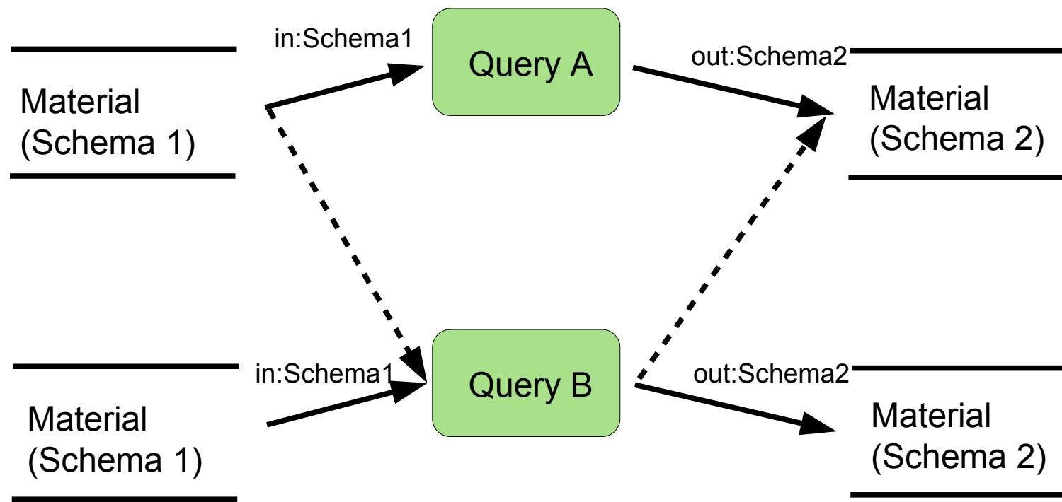
**Tool composition theorem 1:** Two stream-based tools can be composed if their input and output types are compatible and the output order in the output streams is commutative
