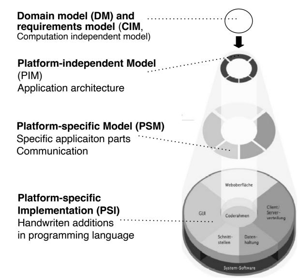
In the MDA, there are **model mappings** between the models DM - CIM – PIM – PSM - PSI
